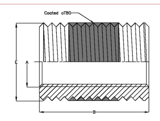
Female thread A = M5Length B= 12.5Male thread E= M7Type= 97x 000 050.100
